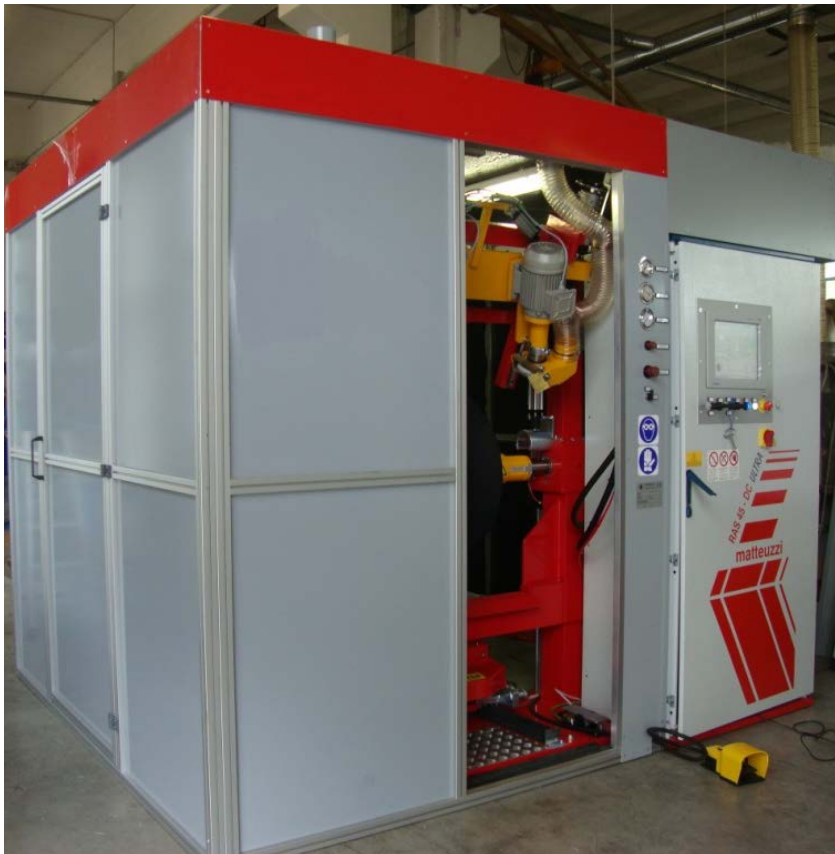
machine complete with sound dampening cabin and automatic front sliding door
